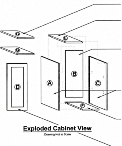
(2-3) Adjustable Shelves. To Be Installed After Assembly and Installation of Finished Cabinet.
